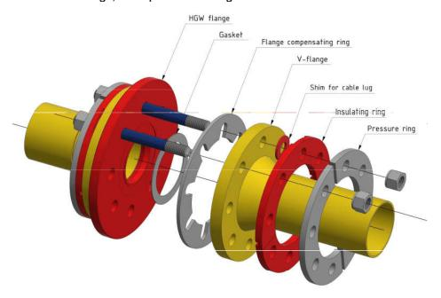
With cable lugs, example 8-hole flange:
