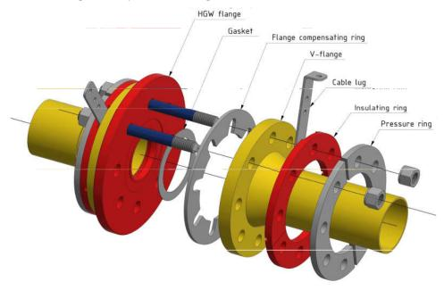
The torque to be applied is indicated in the documentation drawing of the insulating flanges. Stud-bolt with self-lubricating coating.
