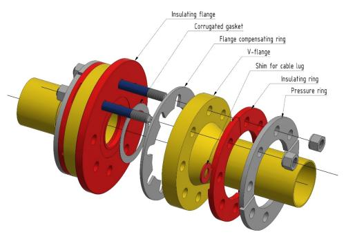
With cable lugs, example 8-hole flange:
