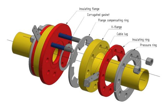
The torque to be applied is indicated in the documentation drawing of the insulating flanges. Stud-bolt with self-lubricating coating.
