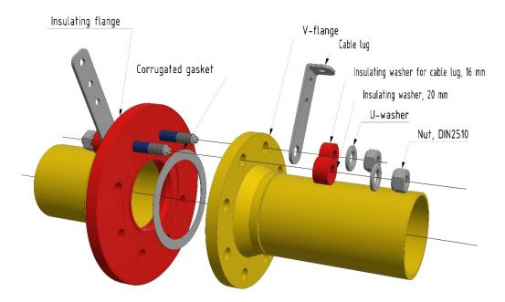
The torque to be applied is indicated in the documentation drawing of the insulating flanges. Stud-bolt with self-lubricating coating.
